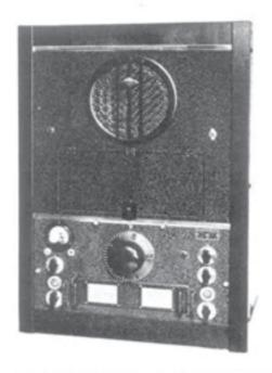
HRO-C -- A Deluxe Receiver Installation consisting of an HRO with an SPC Unit (power unit, coil container and loudspeaker) in an MRR Table Rack. Chromium-plated appearance strips and side trim strips included.
